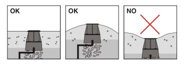
WARNINGS - all enclosures and fittings for external lights must be at least IP65 - allow adequate drainage around fittings.
