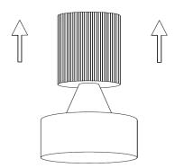
make electrical connections as necessary, pass driver through ring into ceiling void at this time.
