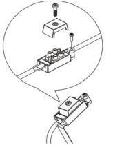
Push fitting up into ring. Fitting will click securely into place.
